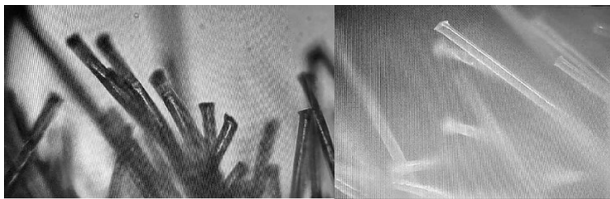
Figure 1 and 2 Nylon hollow fibers at the broken end of test swabs.
